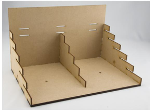
6. Glue the paint shelves into place. Note that the top two have tongues that fit into the rear. Also note how the bottles on alternate shelves are staggered.
