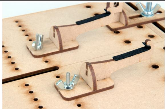
2. The tail plane clamp locates into the long slot at the opposite end of the jig. With the model located against the main plane clamps slide the tail plane clamp up to the tail plane so that the aircraft is held in position. The clamps do not have to be pushed together hard.
