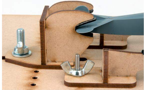
3. The upper wing supports locate into the remaining long slot. Set one of the supports to hold the wing in the required location and then use the graduation markings to set the second support up to match it. It is probably worth using white tack to gently attach the upper wing to the supports.
