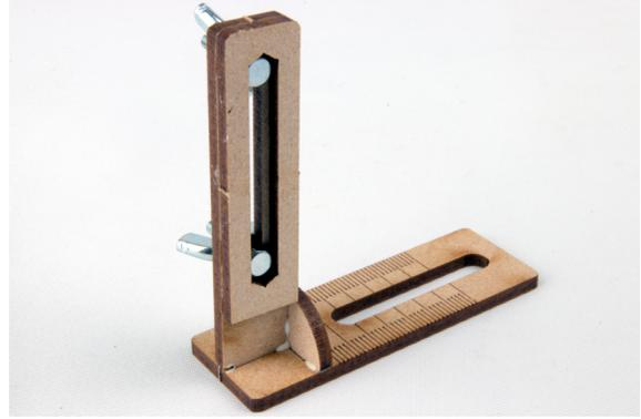
4. The L shaped wing supports bolt onto the uprights with the supports against the graduated face. Do not overtighten the nuts as the wood will distort.
