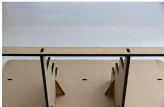
4. Glue the two end verticals into place – slot them into the rear and ensure that they align with the front vertical.
