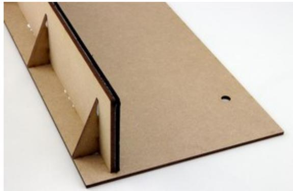
5. Fix the larger neoprene piece to the 3mm base. Place it hard up against the vertical.
