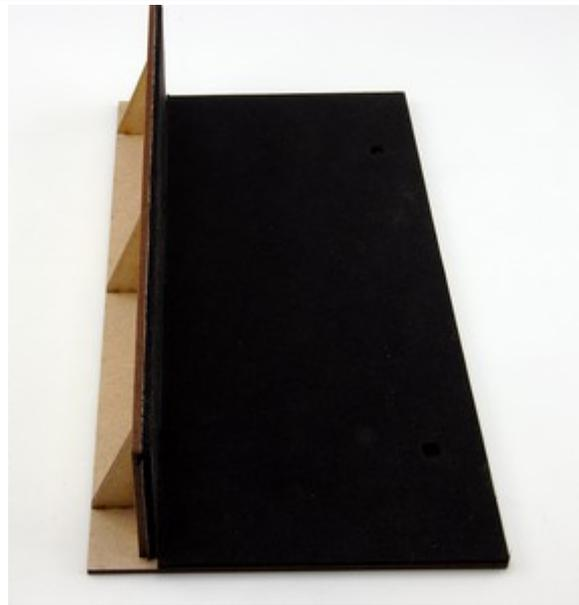
6. Place the two bolts into the hexagonal holes in the 6mm base. Using the bolts to locate the 3mm base glue it to the 6mm base.
