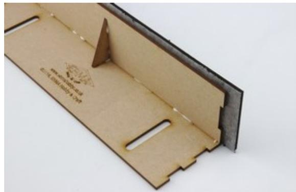
8. Glue the two larger gussetts to the moving piece.
