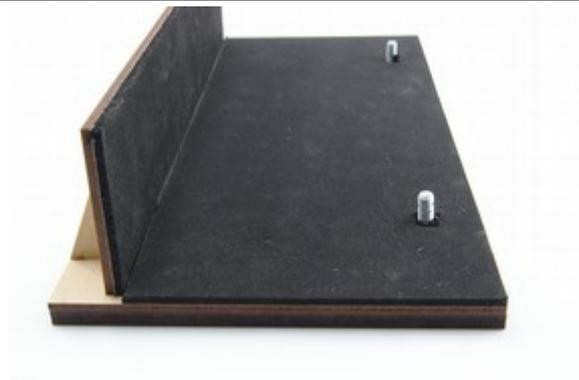
7. Glue the moving vertical to the base piece with the elongated holes. This piece may be used with the logo either face up or down depending on personal preference.
