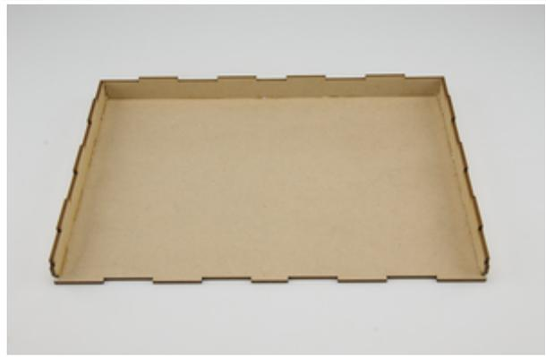
3. Glue the front on. Make sure it is a good joint as you'll be pulling the full weight of the paint with this.
