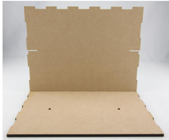
4. Glue the right hand side on. With the sides it is often easier to slide the shelves into the rear and then align with the base.
