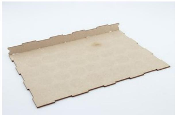
2. Glue the two sides on. Remove any excess glue to ensure that the drawer will run smoothly.
